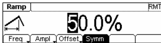
Figure 2-13 Ramp Signal Parameter Setting Interface
