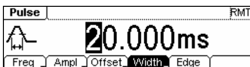
Figure 2-17 Pulse Signal Parameter Setting Interface
